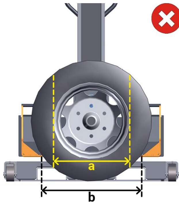
Wheel forks adjusted too far: b > a
